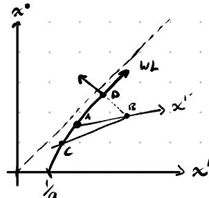
$$\left\{ \begin{array}{l} x^0 = x'' \sinh(ax'') \\ x' = x'' \cosh(ax'') \end{array} \right.$$
