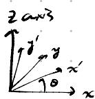
$$\Omega = \begin{pmatrix} c_\theta & -s_\theta & 0 \\ s_\theta & c_\theta & 0 \\ 0 & 0 & 1 \end{pmatrix} \text{ around } \hat{z} \text{ by angle } \theta, \quad \Omega = \begin{pmatrix} c_\theta & 0 & s_\theta \\ 0 & 1 & 0 \\ -s_\theta & 0 & c_\theta \end{pmatrix} \text{ around } \hat{y}$$
