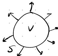
$$\frac{d}{dt} \iiint n dV = - \iiint (\vec{\nabla} \cdot \vec{j}) dV = - \iint_S \vec{j} \cdot d\vec{a}, \quad \vec{j} = \frac{\Delta N}{\Delta A \Delta t} = n \vec{v}$$
